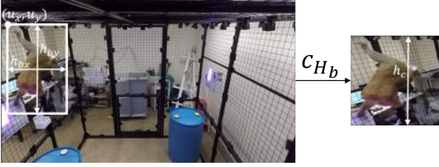
Figure 8: A cropped image is an input to the network where the output is the segmentation distribution with the same size. To rectify the segmentation distribution (heatmap), a series of image transformations need to be applied
