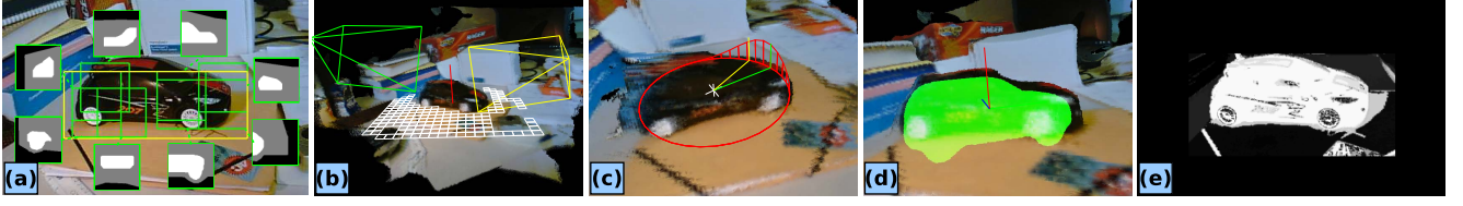
Figure 1. Coarse object pose initialization: (a) Result of the part based detector and related part priors, (b) supporting plane estimation, (c) set of principal angles resulting from the detections (yellow: from detection in first reference, green: second reference) and principal angle interpolation in red, (d) pose from detection, (e) pixel foreground posteriors with which the pose is refined.
