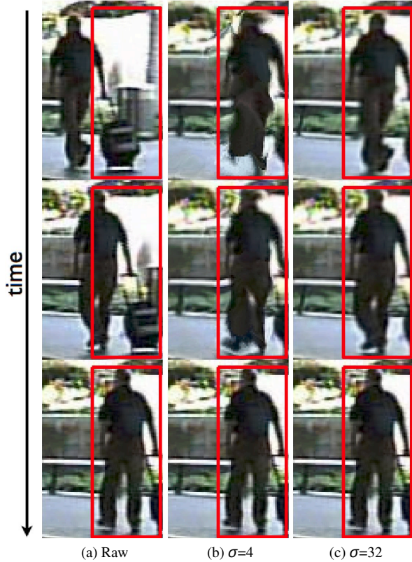
Figure 2: Stabilization using coarse-scale LK flows. We show temporally distant 3-frame sequences stabilized onto the last frame (bottom row). The red box in each frame is the location of the person in the last frame. (a) In the raw video, the person shifts from left to right due to camera and object motion. (b) Using fine-scale LK flows, the overall body is stabilized onto the last frame at the cost of distortion in body parts (most visible at the heads and legs of the top row). (c) Using coarse-scale LK flows the warped images are aligned in terms of the overall body location while still preserving clear motions of body parts.
