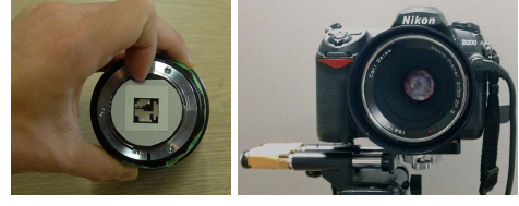
Figure 13. Lens with coded aperture and camera on a slide stage.
