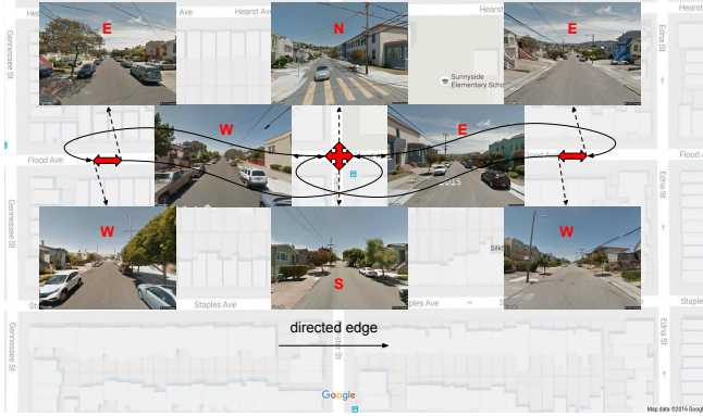
Figure 2: Directed graph illustration. The red arrows represent nodes, encoded by location and direction. Each node has an associated street-view image, taken at the node’s location and pointing in the node’s direction. Nodes are connected by roads (solid connectors in the figure).
