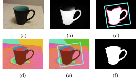
Fig. 4: The minimum enclosing box and homogeneous mask creation process. (a) The model image. (b) The model's saliency map. (c) Automatic thresholding of the saliency map, and the minimum enclosing box (cyan) encapsulating detected contours (pink). (d) The k-means color cluster map. (e) The minimum enclosing box outer lines iterated to obtain the background clustered colors. (f) The final internal homogeneous mask derived by non-background colors within the enclosed box.
