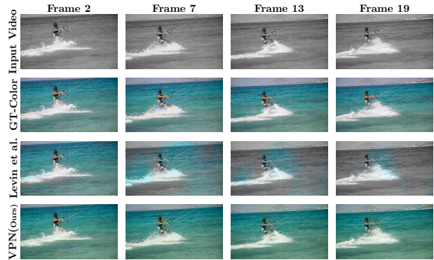
Figure 7. Video Color Propagation. Input grayscale video frames and corresponding ground-truth (GT) color images together with color predictions of Levin et al. [46] and VPN-Stage1 models.
