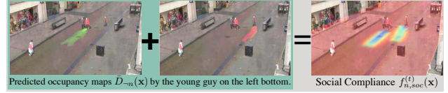
Figure 4. The green box demonstrates how a pedestrian forms beliefs about others \mu_{-n}^{(t)} and encode such information into social compliance feature f_{n,soc}^{(t)}(\mathbf{x}) . Red indicates high reward and blue indicates low reward.
