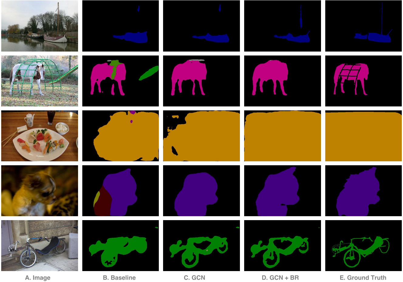
Figure 6. Examples of semantic segmentation results on PASCAL VOC 2012. For every row we list input image (A), 1 \times 1 convolution baseline (B), Global Convolutional Network (GCN) (C), Global Convolutional Network plus Boundary Refinement (GCN + BR) (D), and Ground truth (E).
