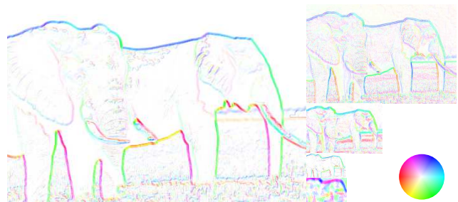
Figure 12. View best in color. Orientated feature maps for the H-DSN. The color wheel shows orientation coding. Note that between layers boundary orientations are colored differently because each feature has a different \beta . This visualization demonstrates the consistency of orientation within a feature map and across multiple layers. The images are taken from layers 2, 4, 6, 8, and 10 in a clockwise order from largest to smallest.
