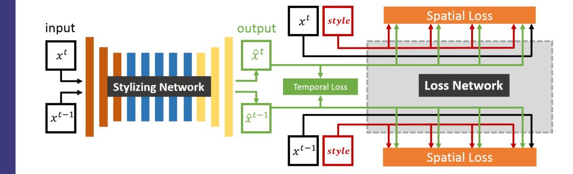
Our style transfer model consists of two parts: a stylizing network and a loss network. The stylizing network takes one frame as input and produces its corresponding stylized output. The loss network, pretrained on the ImageNet classification task, defines a hybrid loss function including spatial and temporal components.
