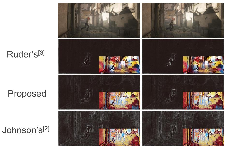
The error maps show the pixel-wise color difference between corresponding pixels of consecutive frames, where the whiter the color is, the larger the error is.
