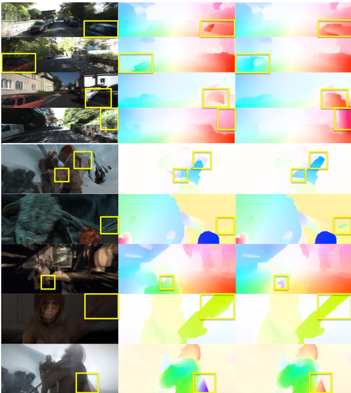
Figure 2. More comparisons to [1]. Left to right: overlapped image pairs, results of [1], results of the proposed method. Details are highlighted using yellow rectangles. Kitti: 1st-4th row; Sintel: 5th-9th row.
